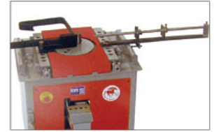
STIRRUP ACCESSORIES Optional, stirrup bending tool & adjustable length stop
