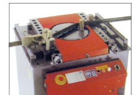
LEFT/RIGHT STANDARD Produce Double Bends and bend from Left to Right
