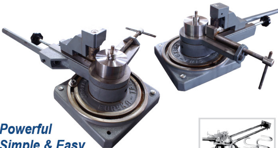
"S" SCROLLS Shown with Optional Bar Brake / Folding Tool
