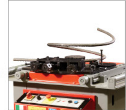
HEAVY DUTY SPIRAL DEVICE OPTIONAL Use with up to #6 Bar
