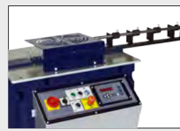
STIRRUP ACCESSORIES Optional, stirrup bending tool & adjustable length stop
