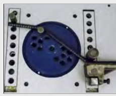
LEFT/RIGHT STANDARD Produce Double Bends and bend from Left to Right
