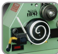
Easy Ratchet Lateral Guide Adjustment
