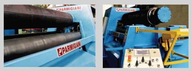
PARMIGIANI LINEAR GUIDES: Minimum bending diameter up to 1.1 x top roll diameter.
