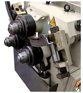
Lateral guides used for angle leg-in
