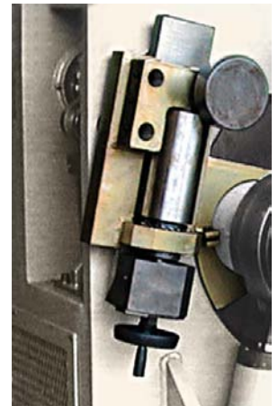
Tri-directional lateral material guides standard Tri-directional hydraulic powered: 308 - 315
